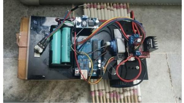
**Fig 3: Physical Prototype of the TSA System**
