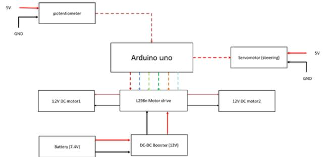
Fig 2: System Hardware Architecture
