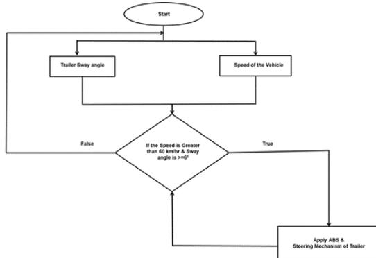
Fig 1: Process Flow Diagram of the TSA System
