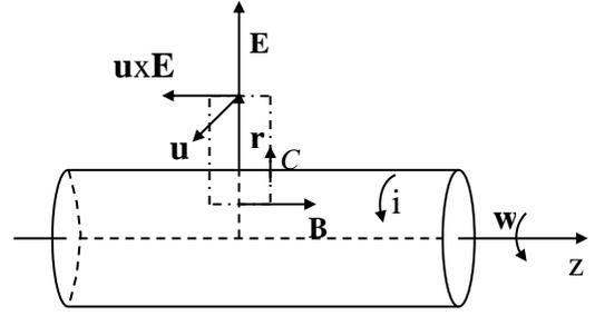
Figure (3.6). The fields  $\mathbf{u} \times \mathbf{E}$  and  $\mathbf{B}$ , the curve  $C$ , and the linear current density  $i$  for the rotating charged cylindrical shell with angular velocity  $\omega$ .
