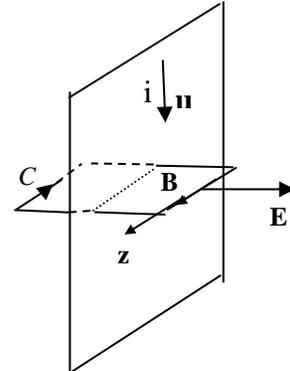
Figure (3.5).  $\mathbf{B}$  field line, curve  $C$ ,  $\mathbf{u}$ , and the direction of the planar current distribution  $i$ .
