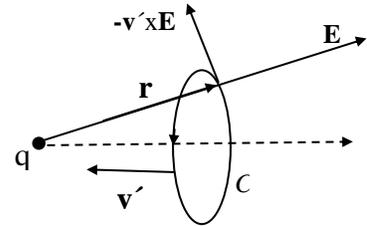
Figure (4.3). Curve  $C$  with velocity  $\mathbf{v}'$ , coinciding with the field lines  $-\mathbf{v}' \times \mathbf{E}$  and  $\mathbf{B}$ , and the charge at rest.
