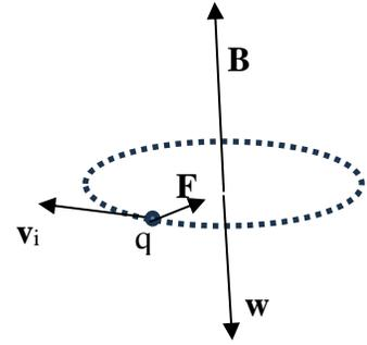
Figure (4.1). Path of a particle with charge  $q_i$  in a uniform magnetic field  $\mathbf{B}$ .
