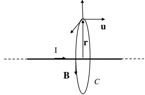
Figure (3.1) Speed  $\mathbf{u}$  of the electric field line  $\mathbf{E}$  at point  $\mathbf{r}$ , due to the charge carriers in the infinite straight wire. The field lines  $\mathbf{u} \times \mathbf{E}$  and  $\mathbf{B}$ , coinciding with curve  $C$ , are also shown.
