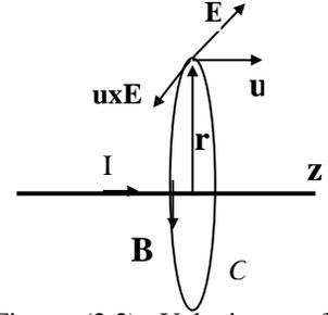
Figure (3.3). Velocity  $\mathbf{u}$  of the  $\mathbf{E}$ -field lines at  $\mathbf{r}$ , and the lines of the  $\mathbf{u} \times \mathbf{E}$  and  $\mathbf{B}$  fields coinciding with curve  $C$ .
