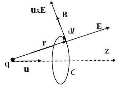
Figure (3.2). Fixed circular curve  $C$ , coincident with the lines of the fields  $\mathbf{B}$  and  $\mathbf{u} \times \mathbf{E}$ , element  $d\mathbf{l}$  at position  $\mathbf{r}$ , charge  $q$  with velocity  $\mathbf{u}$  along the  $z$ -axis direction.
