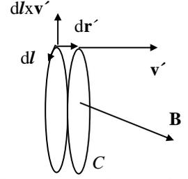
Figure (1.1). Circuit  $C$  with velocity  $\mathbf{v}'$  in the magnetic field  $\mathbf{B}$ .
