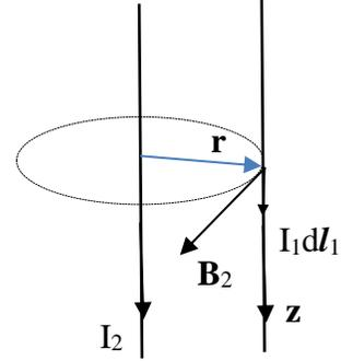
Figure (4.2). Some quantities used in calculating the magnetic force between two long current-carrying wires.
