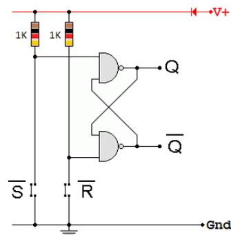
Figure 6: Bistable Latch: pair of NAND gates
