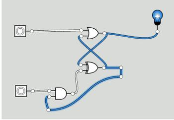
Figure 7: Simulated Tononi circuit on logic.ly
