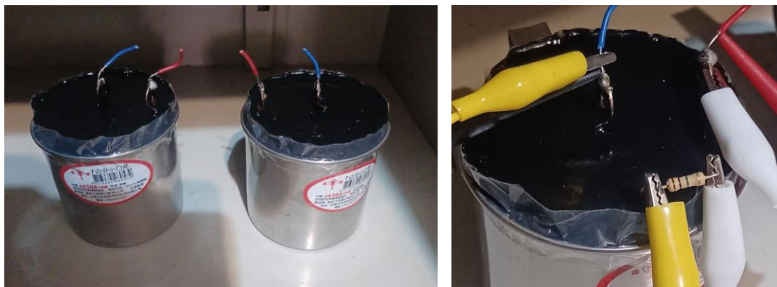
Fig. 8. Selected images of the gravity battery during the static measurement process.
