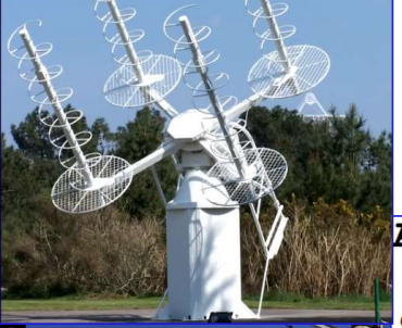
Circularly polarized light can be generated using helical antenna
