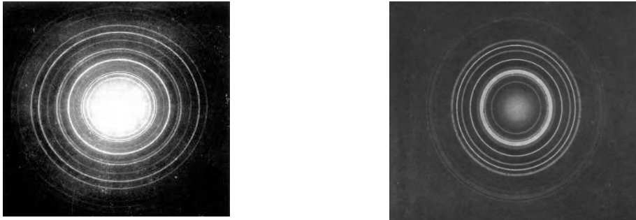
Fig. 28. Experimental electron diffraction patterns obtained as a result of electron diffraction on the surface of crystals
