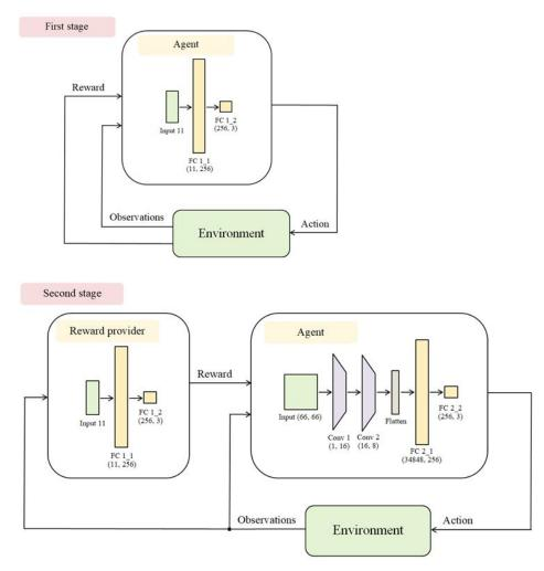
Figure 16: Mechanism of complexification through reward providing
