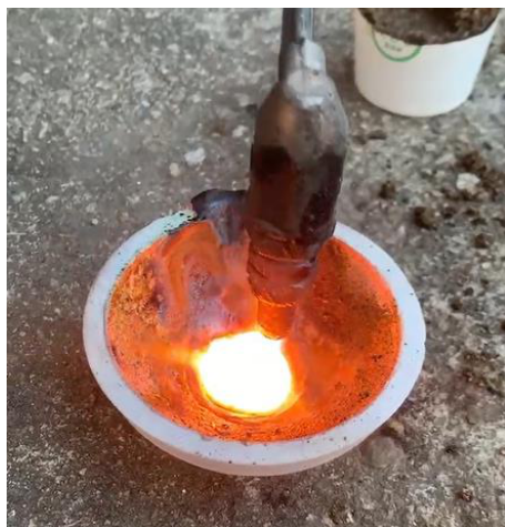
Fig. 1. Heat treatment process of the Pb-Cu-P-S-O compound using oxygen-cutter.
