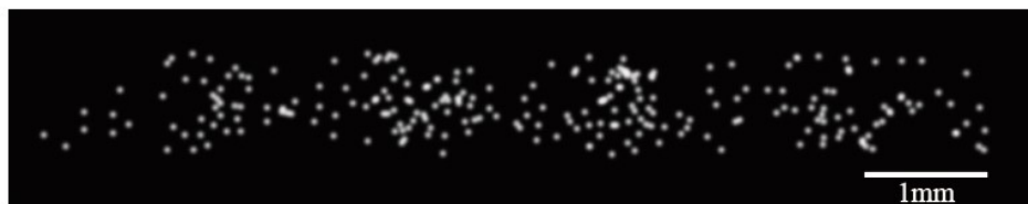
Fig. 4. The image was obtained by superimposing the photon positions after imaging the multiple reflection interference light 100 times with the ICCD (each photon was drawn with the same luminance). Interference fringes due to photons can be observed.
