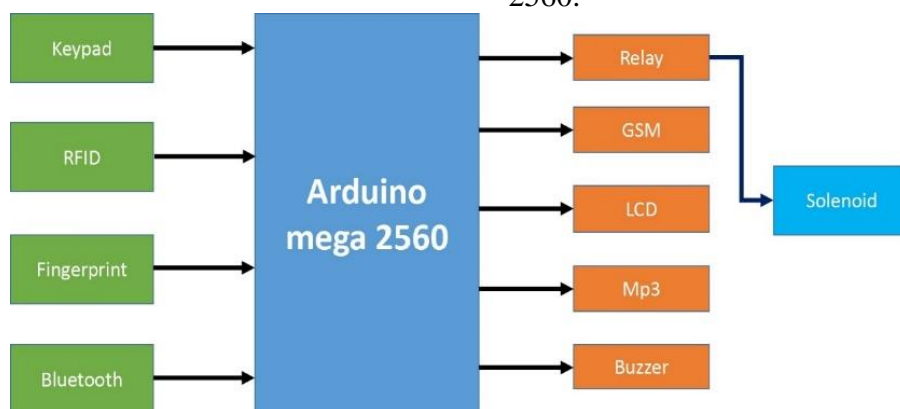
Figure 6. Configuration diagram of the quadruple security system
