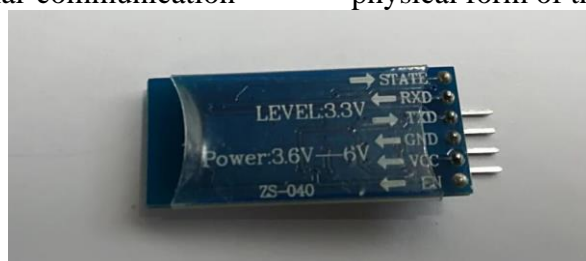
Figure 13. Physical form of Bluetooth HC 06
