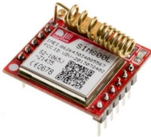
Figure 14. Physical form of SIM800 GSM module
