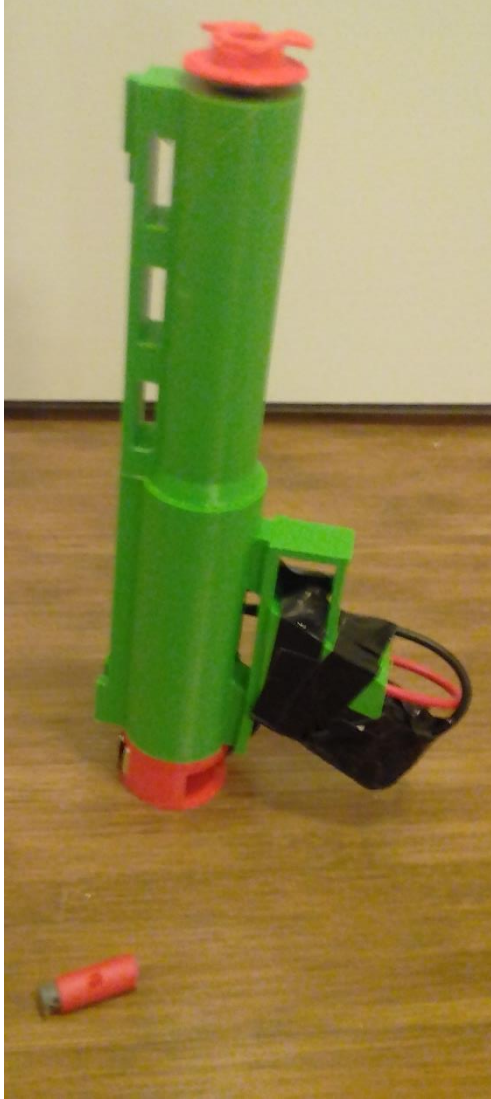
Figure 13: Lachesis prototype 2 with projectile, thicker wire, and muzzle-mounted line spool.
