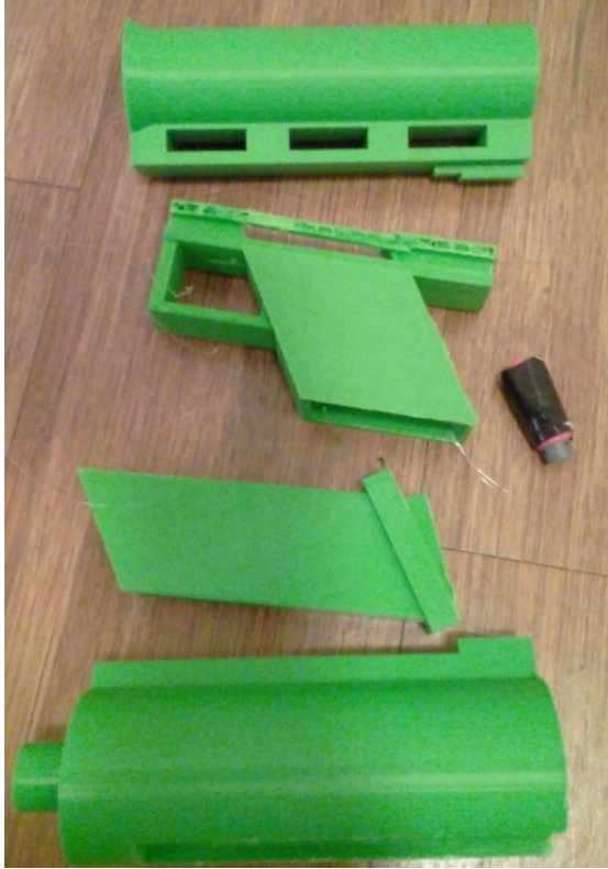
Figure 7: Primary 3D printed prototype components including barrel, grip, magazine, and projectile.
