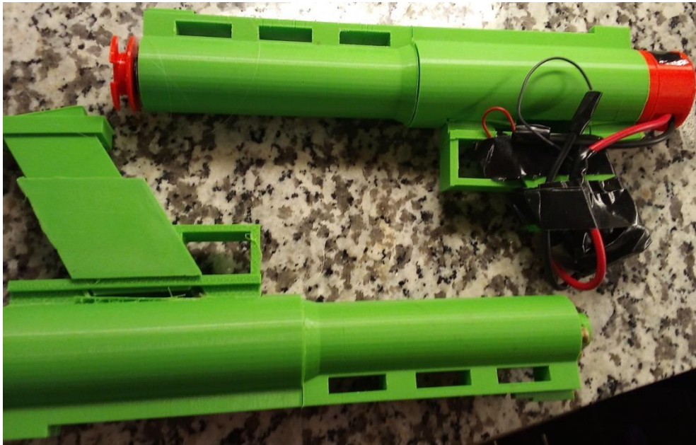
Figure 15: Two prototype line launchers, with Prototype 1 on bottom and Prototype 2 on top.
