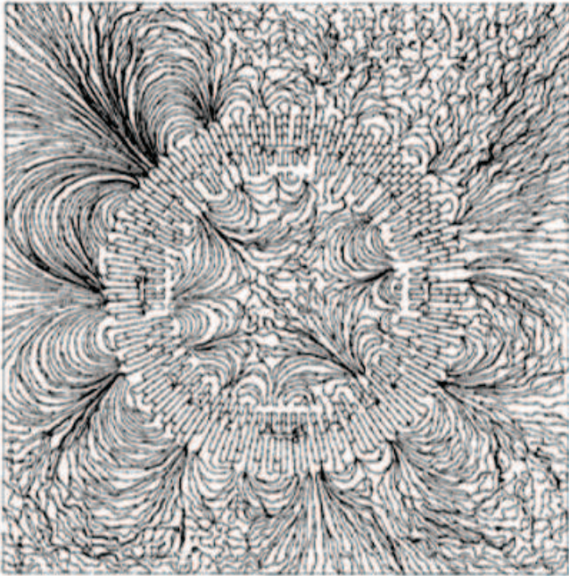
Fig. 1. Distribution of vorticity (vortex lines) in the plane of 80-vorton ring.
