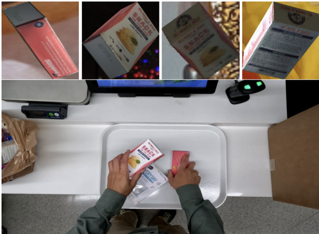
Figure 3. The proposed pipeline. In the first stage, a class-agnostic detector proposes boxes for cropping products. Then, a classifier categorizes corresponding classes of patches. Lastly, a tracker link predictions across frames to form the final result. [14]
