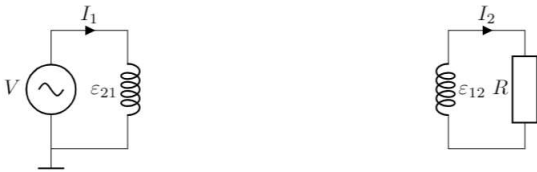
Fig. 3. When the secondary coil moves to a place far away from the primary coil, in fact, the primary coil becomes a transmitting antenna and the secondary coil becomes a receiving antenna.
