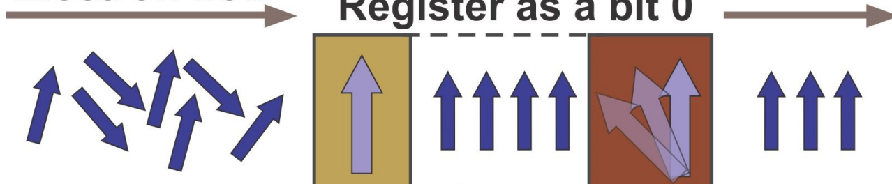
Figure 5: Polarization fields aligning spins of the electron flow. Magnetic resistance on tunneling, an electric current flows easily, through the two magnetic configurations that lead to spins with the same sense and showing resistance when opposite spins senses result from differently oriented magnets.
