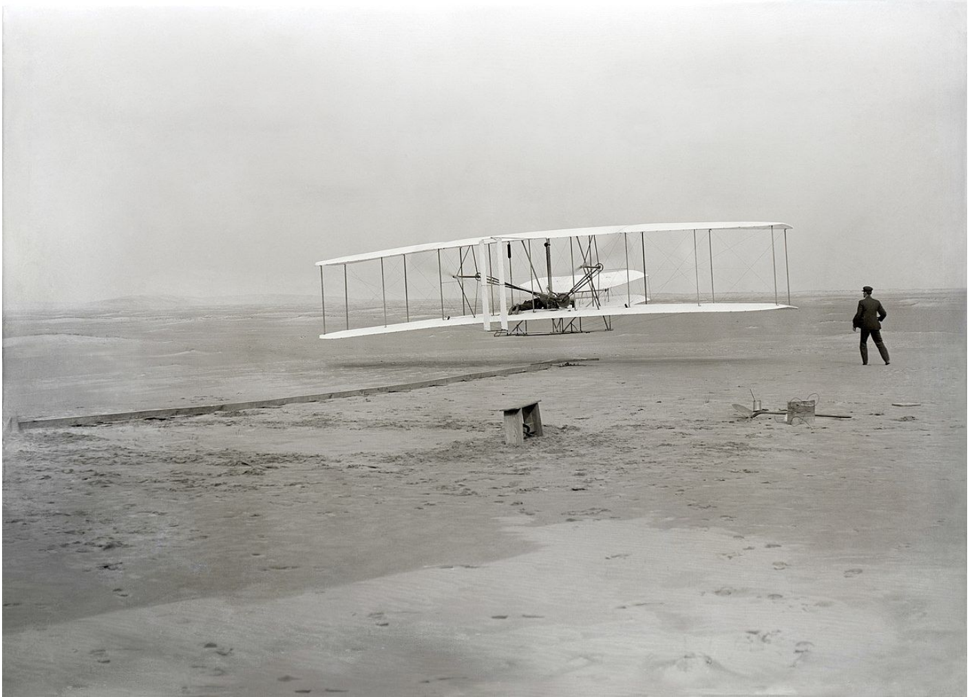
Figure 1: The first powered, controlled, sustained airplane flight in history. Orville Wright, age 32, is at the controls of the machine, lying prone on the lower wing with hips in the cradle which operated the wing-warping mechanism. His brother, Wilbur Wright, age 36, ran alongside to help balance the machine, having just released his hold on the forward upright of the right wing. The starting rail, the wing-rest, a coil box, and other items needed for flight preparation are visible behind the machine. (Orville Wright preset the camera and had John T. Daniels squeeze the rubber bulb, tripping the shutter) Data and picture courtesy: John T Daniels, Wikipedia.
