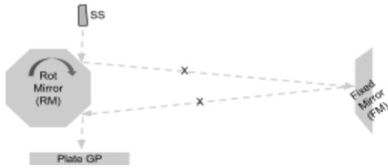
Fig 4. Modified Facault's setup. A polygonal mirror with a considerable radius replaces a rotating mirror. But this setup is unable to record any SILT advantage.
