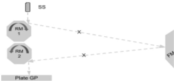
Fig 5. Schematics of lightspeedometer. The 'X' distance between RM and FM is larger and is not shown up to scale.
