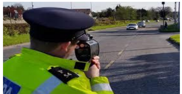
Radar gun used for monitoring car speed
