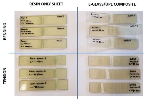
Figure 1. All four classes of samples after mechanical testing was performed.
