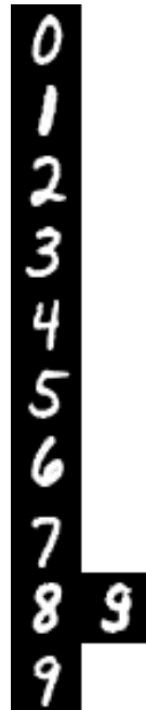
Fig.14 Incorrect case of ICGC prediction. \sigma = 0.0 . Number 9 on the right side is the input image but ICGC predicted number 8.
