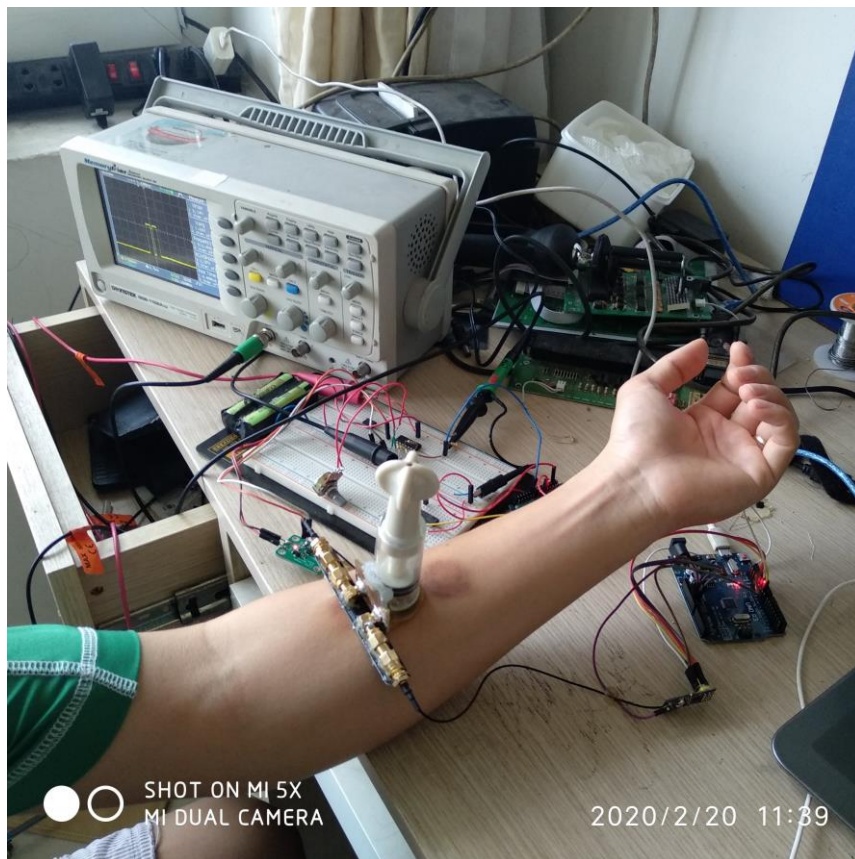
Fig. 3.1. Measurement setup using the proposed glucose sensor.
