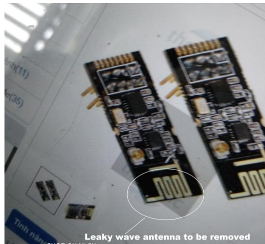
Fig. 2.2. RF/microwave Transmitter generating an RF at 2.4 GHz.
