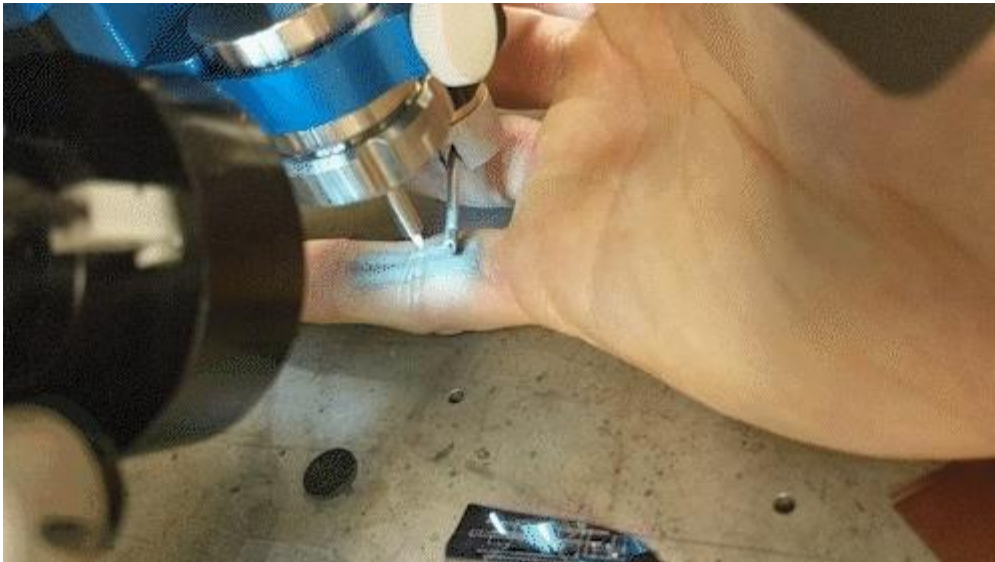
Duke graduate student Nick Williams prints two electronically active leads along the underside of his pinky finger, places small LED light between them, and applies a voltage to show the circuit stays intact even when he bends his finger. Credit: Nick Williams, Duke University
