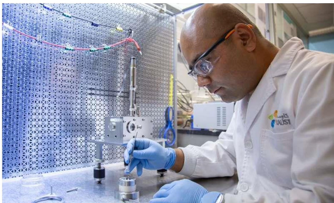
Buddha Shrestha loads a silica disk with an ultrasmooth-surface terminated with per fluorocarbons comprising 10 carbon atoms. Credit: © 2019 KAUST
