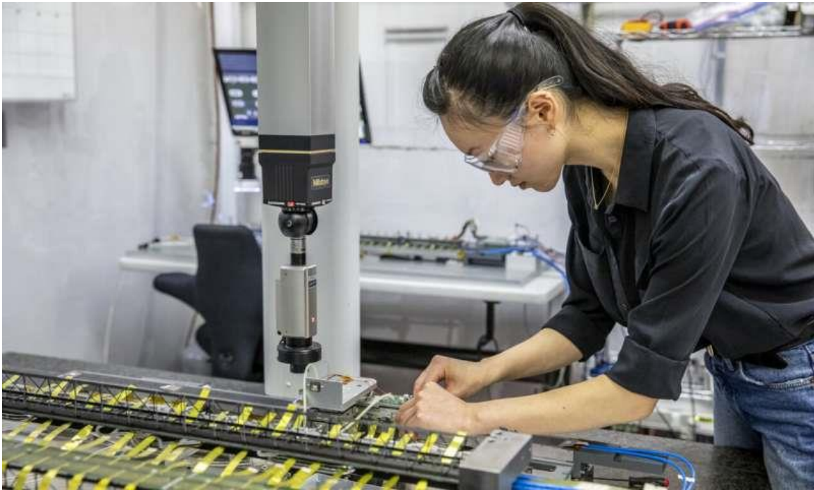
Berkeley Lab's Erica Zhang conducts measurements of a detector stave during assembly. Credit: Marilyn Chung/Berkeley Lab
