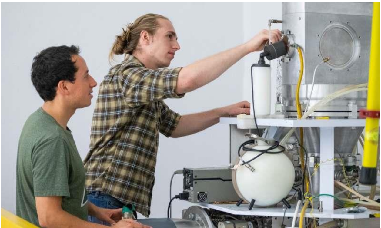
Graduate students Mauricio Ayllon Unzueta (left) and Jonathan Morrell adjust the high flux neutron generator in an underground vault at UC Berkeley. The aluminum vacuum chamber contains the deuterium plasma and the cathode target where the neutrons are generated via fusion. Credit: UC Berkeley photo by Irene Yi
