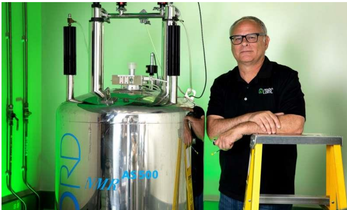
Salk Professor Joseph Noel, pictured in his lab, next to an NMR spectroscopy machine, which is used to decipher the detail of the electronic structures of molecules. Credit: Salk Institute
