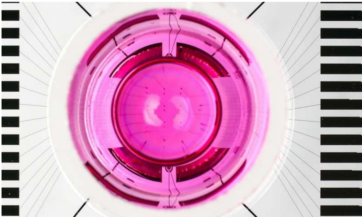
A nanovolcano array with a cell culture ring mounted on a microchip. Credit: A.Herzog/EPFL
