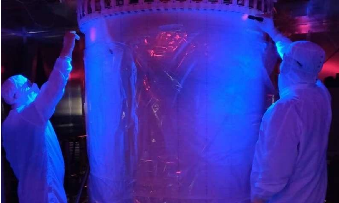
The detector is inspected under UV light. Credit: Nicolas Angelides
