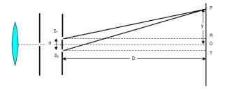
FIG. 1. Double Slit Interference
