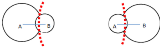
Figure 5. Locus of the points of intersections of two uniformly expanding circular wavefronts is a branch of a hyperbola (red dotted line). When source center A emanates a wavefront before B, the right hyperbolic branch is formed and when B emanates before A, the left hyperbolic branch is formed.
