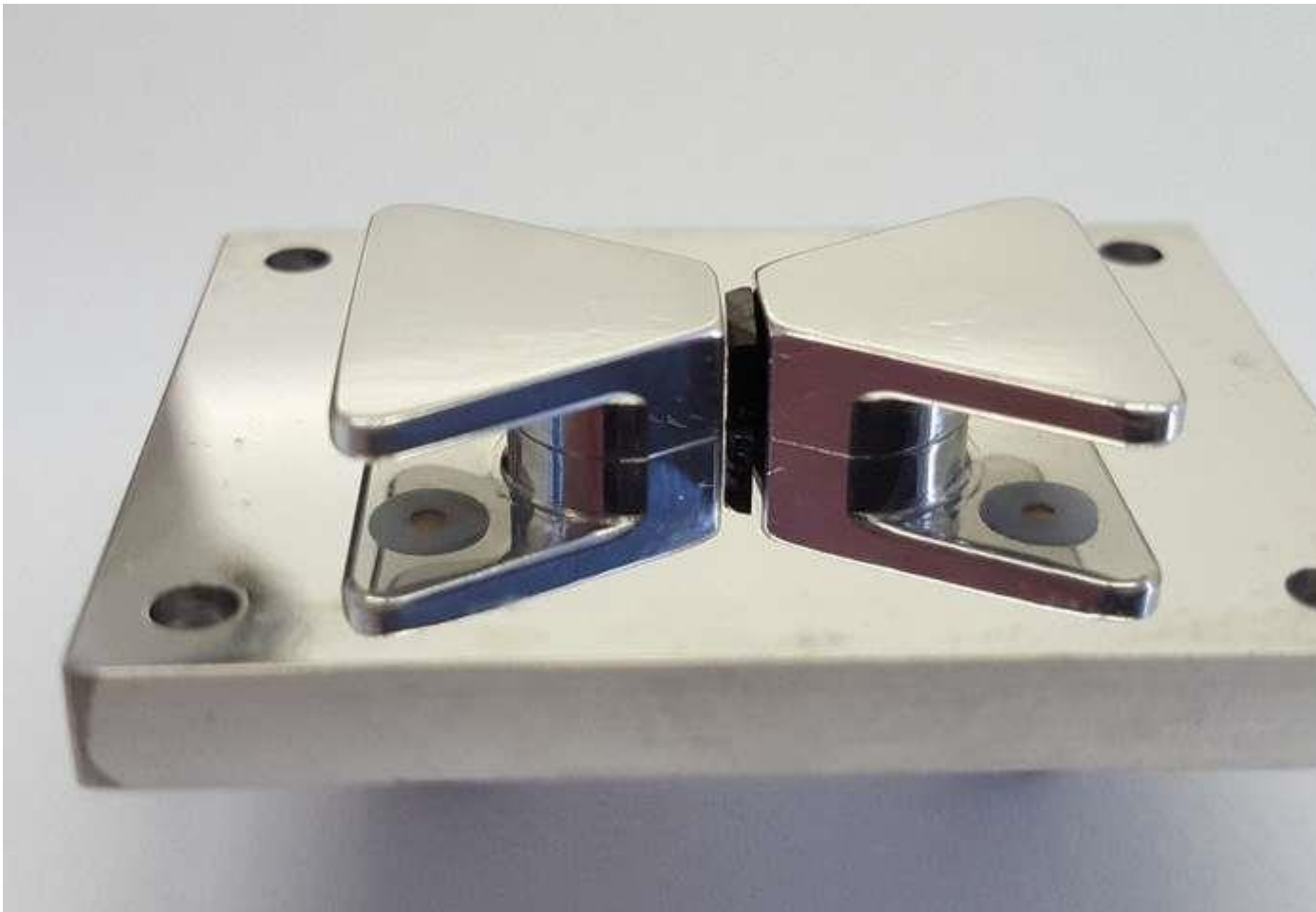
The microwave resonator with the diamond in the middle. Because of the lattice defects, the diamond is black. Credit: Vienna University of Technology
