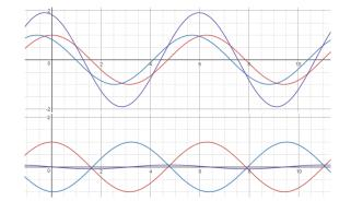
Figure 5: Constructive and destructive interference for linearly polarized beams
