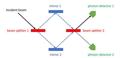
Figure 4: The Mach-Zehnder interferometer
