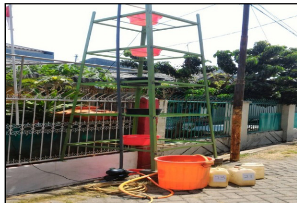
Fig. 1. Multiple Tray Aerators
