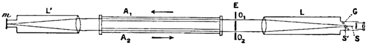
Figure 4: Original layout of Fizeau's experiment
