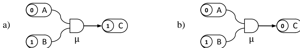
Fig. 3: The logic gate representing the AND operation: a) Toma A is in state 0, tomas B and C are in state 1. The function \mu is \theta[C_{\#}] := \theta[A_{\#}] \wedge \theta[B_{\#}] . b) When \mu is selected for an update, this function is evaluated and the state of toma C changes to 0.
