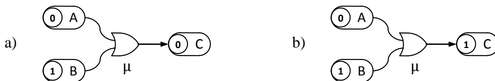
Fig. 4: The logic gate representing the OR operation: a) Toma B is in state 1, tomas A and C are in state 0. The function \mu is \theta[C_{\#}] := \theta[A_{\#}] \vee \theta[B_{\#}] b) When \mu is selected for an update, this function is evaluated and the state of toma C changes to 1.
