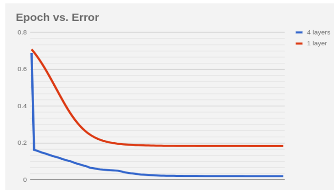
Fig. 4. Error using 1 layer and 4 layers fully connected Neural Networks trained through 1000 epochs. 1 layer error: 0.175971; 4 layers error: 0.012657
