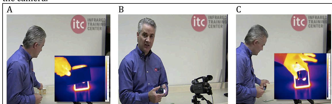
Figure 14. Non Thermoelectric Germanium. (A) 'Opaque' thermoelectric glass in front of the heat source; (B) visibly opaque germanium in hand; (C) 'transparent' non-thermoelectric germanium placed in front of heat source [41].
