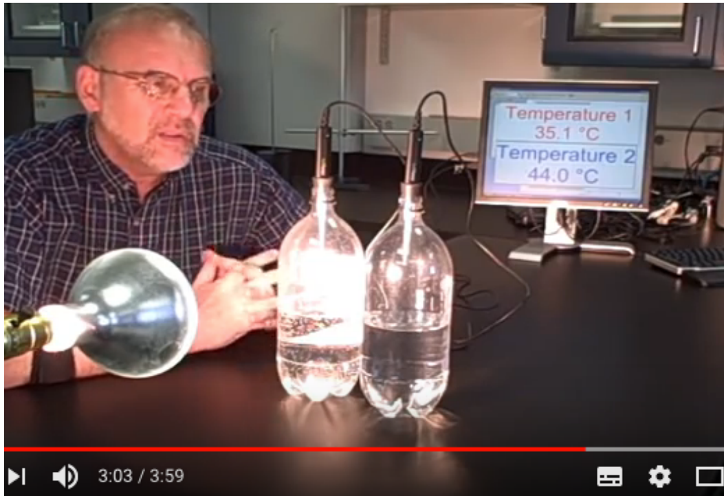
Figure 47. Greenhouse Gas Bottle Demonstration [62]. Bottles with CO 2 and air are radiated and temperature measured – CO 2 in blue. Is this not an experiment to measure the heat capacities of the respective gases?
