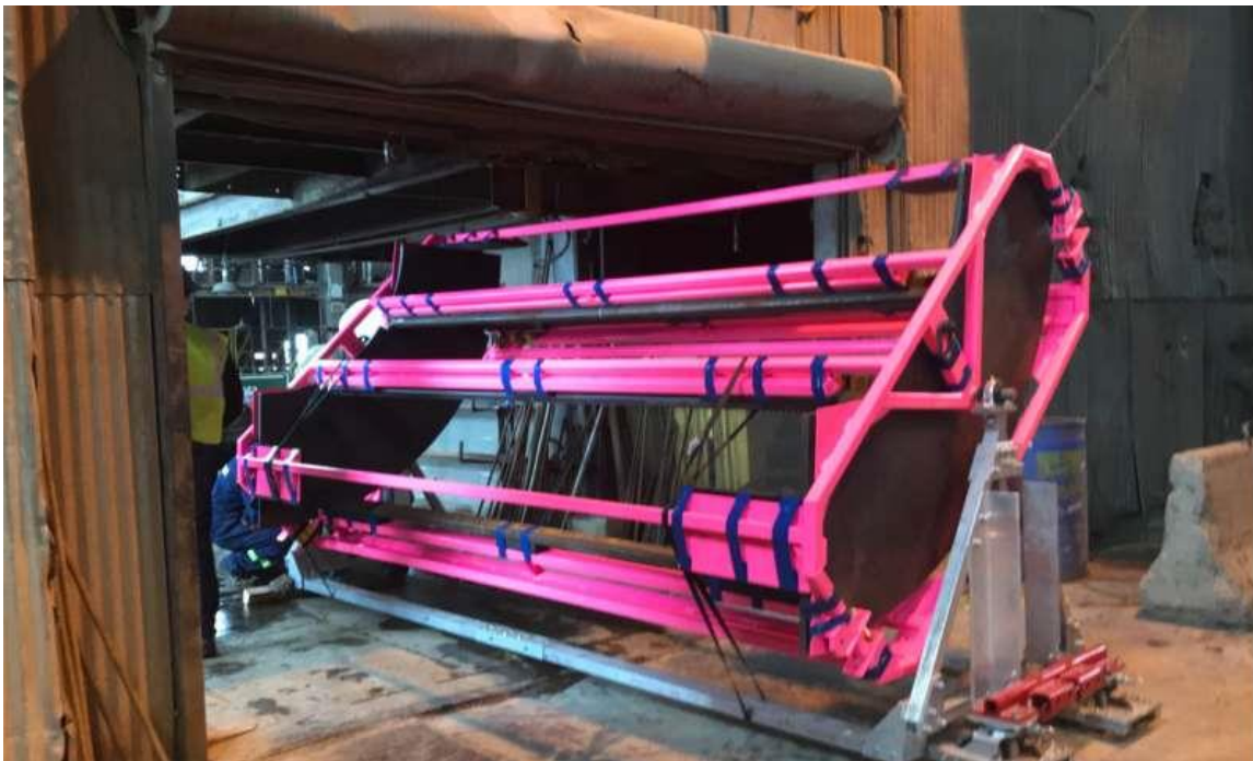
A sturdy, custom-designed pink frame holds one of the 12-foot-tall acrylic tanks. Credit: LZ Collaboration
