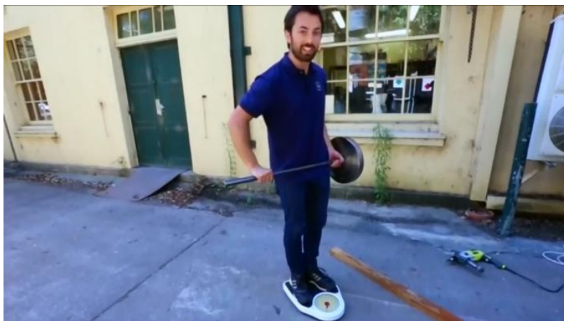
Fig. 6. Muller stands on the scale, holding the non-rotating gyroscope with two hands
