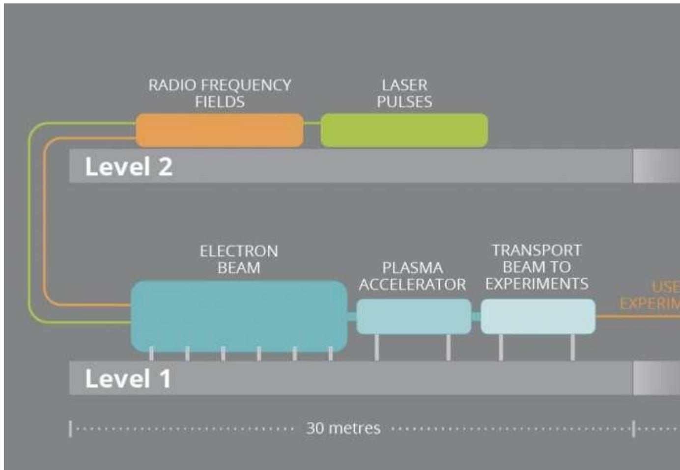
A two-storey design limits the length of the 5 GeV EuPRAXIA plasma accelerator facility, although it could extend to 35-250m depending on what applications are added downstream. Diagram not to scale. Credit: Horizon
