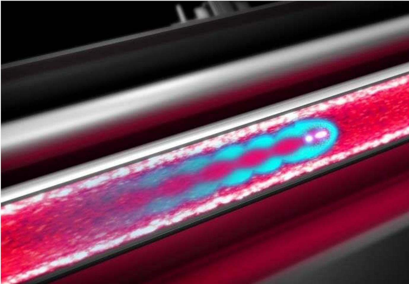
Researchers will use FACET-II to develop the plasma wakefield acceleration method, in which researchers send a bunch of very energetic particles through a hot ionized gas, or plasma, creating a plasma wake for a trailing bunch to “surf” on ...[more](#)
