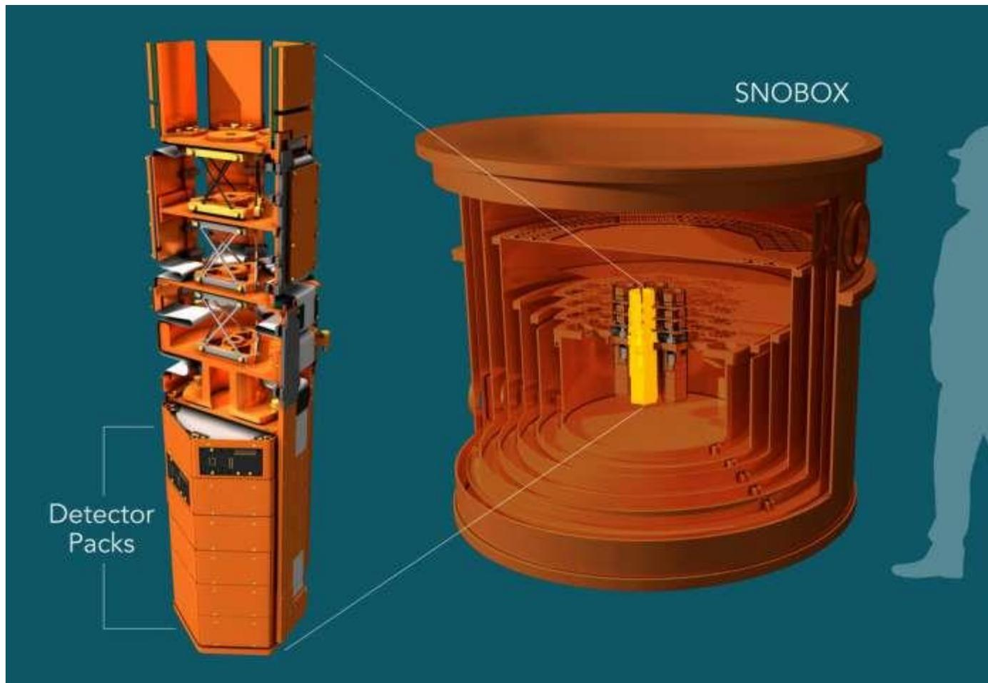
The centerpiece of the SuperCDMS SNOLAB experiment will be four detector towers (left), each containing six detector packs. The towers will be mounted inside the SNOBOX (right), a vessel in which the detector packs will be cooled to almost ...[more](#)
