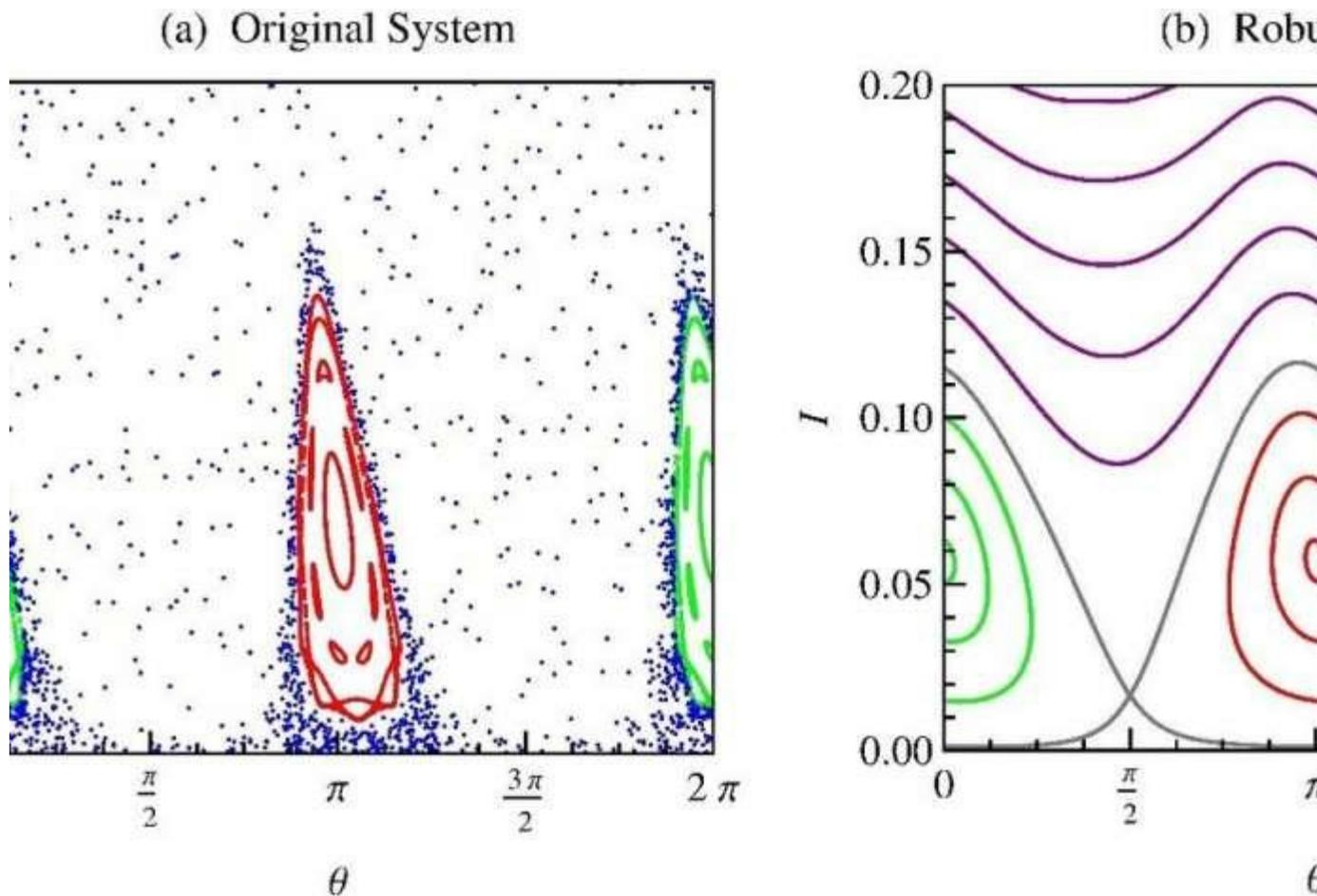
The image compares particle trajectories without (left-hand) and with (right-hand) the presence of the transport barrier. The vertical axis is proportional to the energy of the particles in the accelerator. The blue dots in the left-hand ...[more](#)
