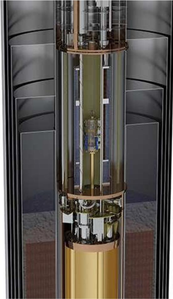
A cutaway rendering of the ADMX detector, which can detect axions producing photons within its cold, dark interior. Credit: ADMX collaboration
