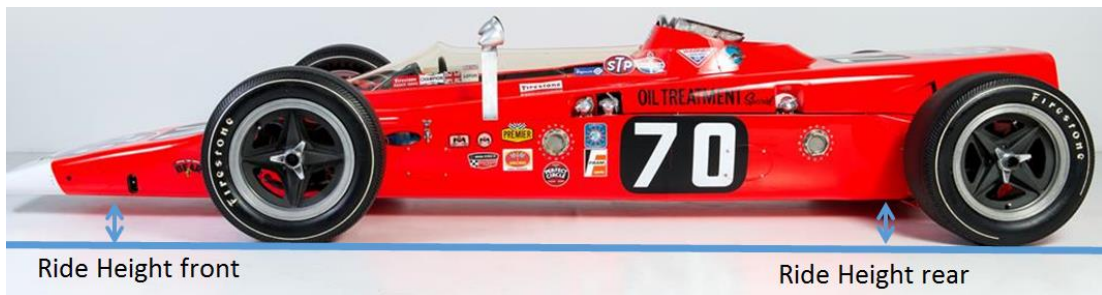
Fig.57: Car freedom degrees / movements in every axes; Ride heights.
