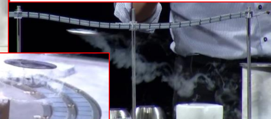
Magnetic field is QUANTIZED inside the superconductor.
