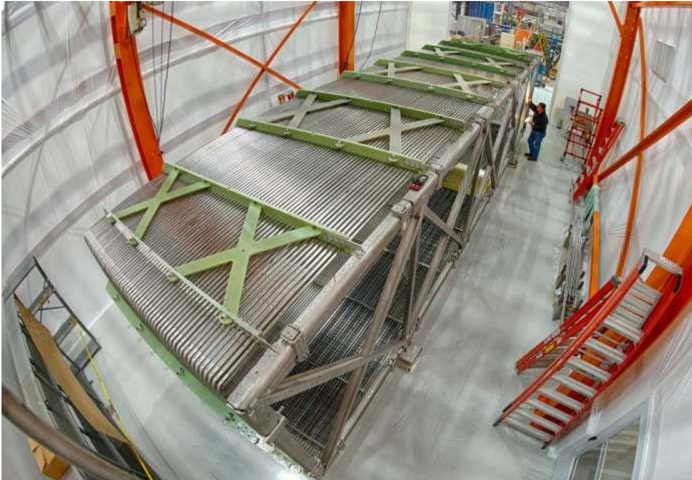
The school-bus-size MicroBooNE Time-Projection Chamber. Credit: Fermilab
