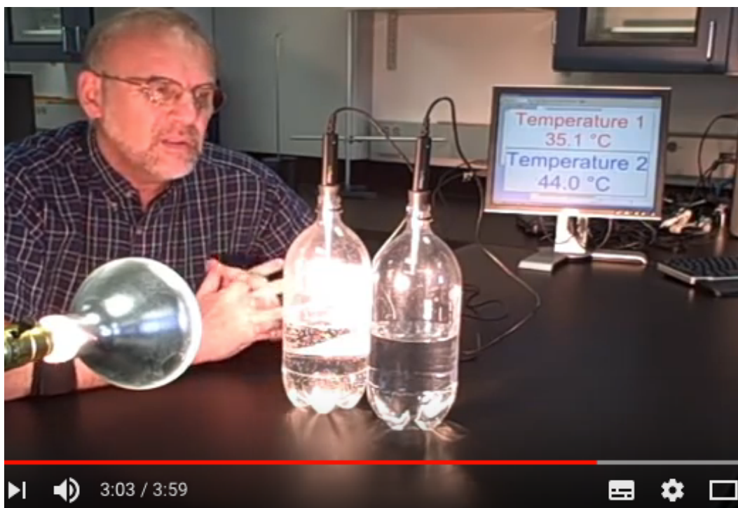
Figure 56. Greenhouse Gas Bottle Demonstration [97]. Bottles with CO 2 and air are radiated and temperature measured – CO 2 in blue. Is this not an experiment to measure the heat capacities of the respective gases?
