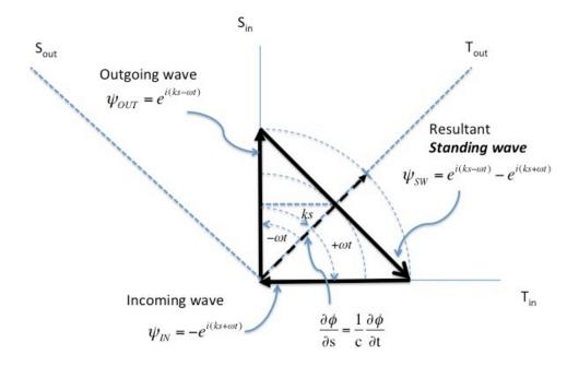
Figure 2 Resultant standing wave vector is the sum of the outgoing wave and incoming wave
