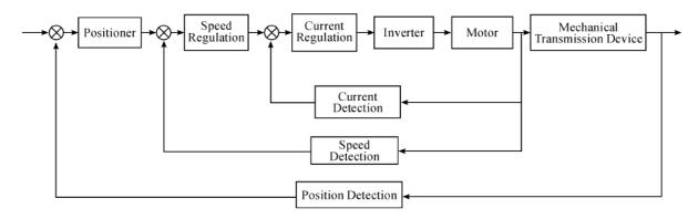
Fig.1 The structure diagram of the CNC machine tool feed system
