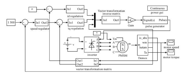
Fig.2 The simulation model of PMSM vector control system
