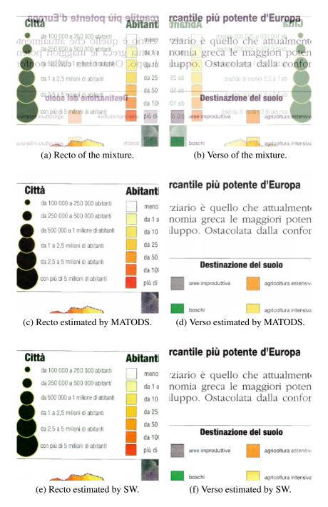
Figure 29: Document in Figure 13 mixed with a mixture matrix as in (69).
