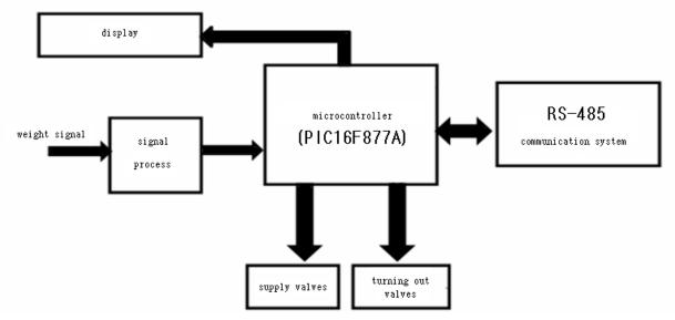
Figure 2. Block diagram of the of the determination feeder for the cosmetics batch
