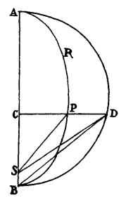
Fig. 2. ADB is a semicircle, ARPB forms an elliptic arc, with particle at P. S is the focus, and AB = 2a.
