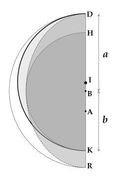
Fig. 1: Circle *DK* (bold line) centered on *I* is the "arithmetic mean," BD = a and BK = b, and *DR* (dashed line) is the ellipse. *A* is the focus of the orbital movement.
